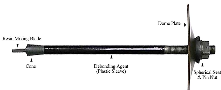
Figure 9. Modified cone bolt.
