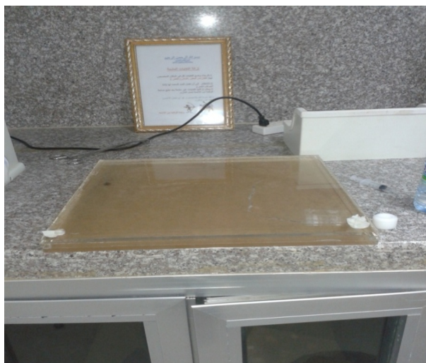
Figure 2. The back part simulates the liquid flood phantom made of Perspex ( 42 \times 42 \times 1 cm) and has orifice 0.5 cm to be fill with a liquid radioactive material.
