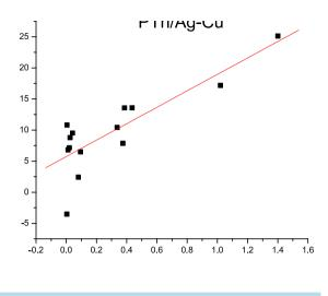
**Figure 4.** PTh-Ag  $\ln \sigma_0$  vs  $E_a$  plots. The MN rule is not fulfilled for samples with *x* upper  $x_c$  (percolation threshold fraction).
