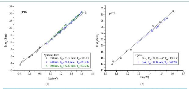
**Figure 3.** (a) pPTh  $\ln \sigma_0$  vs  $E_a$  plots. The data are plotted in heating-cooling cycles for polymers synthesized at 150, 240 and 300 min of reaction, (b) first and last heating cycles for all synthesis times. A good agreement with the MN rule is observed.
