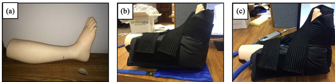
Figure 1. Orientation of control pressure mapping. (a) Manikin leg; (b) The leg is placed in the boot and set atop the Sensor Edge pressure mapping pad to gain an understanding of contact forces existing between surfaces; and (c) The sensor grid is wrapped around the heel and inserted into the boot to gain total heel contact measurements.
