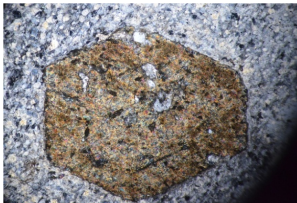
Figure 13. Amphibole phenocrysts in dacite (field length: 1.8 mm, 100X) (XPL).
