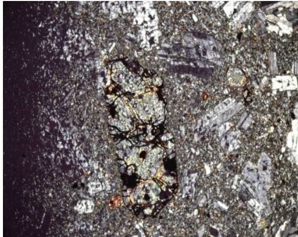
Figure 5. Skeletal structure as result of epastrization of grains of olivine in basalt rocks with serpantinization phenomena (field length: 4.5 mm, 40X) (XPL).
