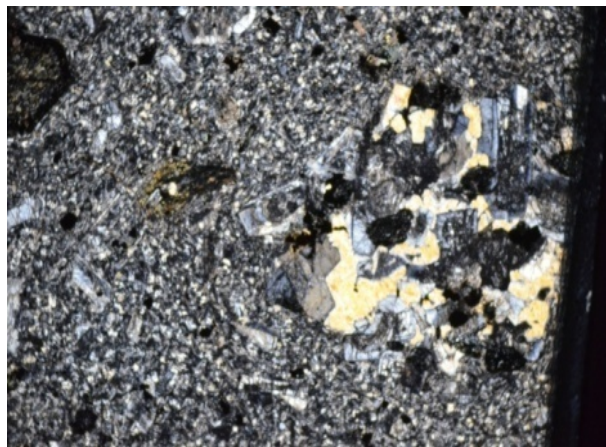
Figure 12. Granite micro enclaves in the andesitic rocks (field length: 4.5 mm, 40X) (XPL).
