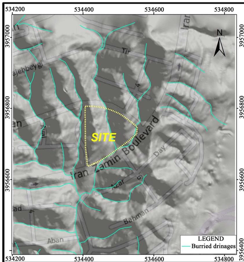
**Figure 5.** A part of aerial photograph related to 1963 from the site of Iranzamin construction project in the Shahrak-e Ghods, Tehran that shows dendritic drainage pattern of Darakeh stream.
