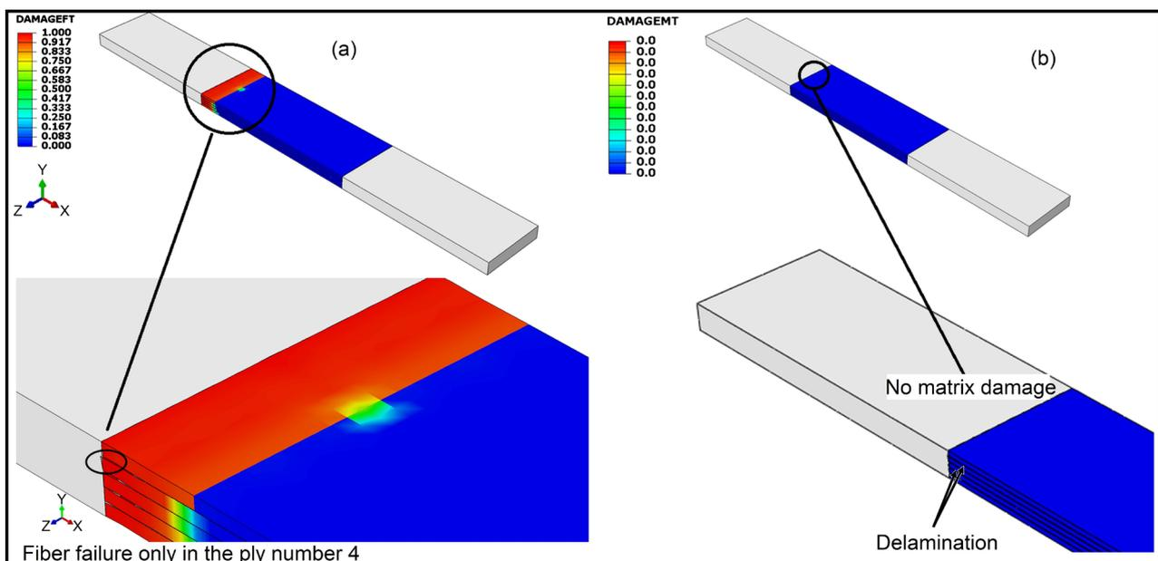
Figure 12. Contour plots (a) (b) showing detection of the final fracture of the YS90A composite under tension.
