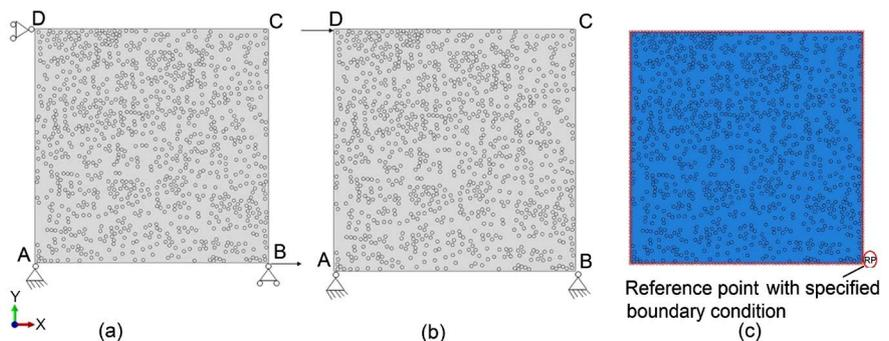
Figure 1. Representation of the periodic boundary condition in tensile (a) and shear (b) loading scenarios.
