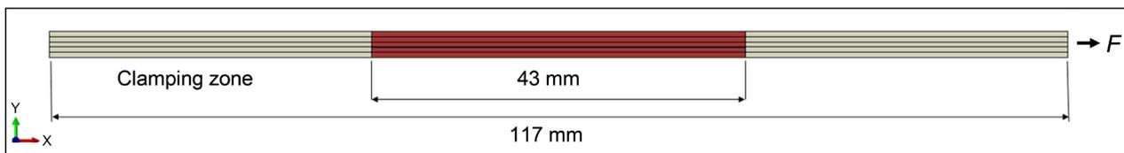
Figure 6. Finite element model representing the laminate and cohesive zone modeling for the on-axis tensile and bending.
