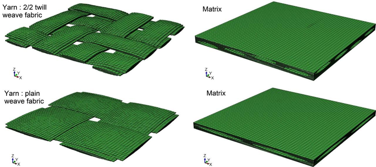
**Figure 2.** FEM Model developed in TexGen with the 2/2 twill weave and the plain weave reinforcement fabrics.
