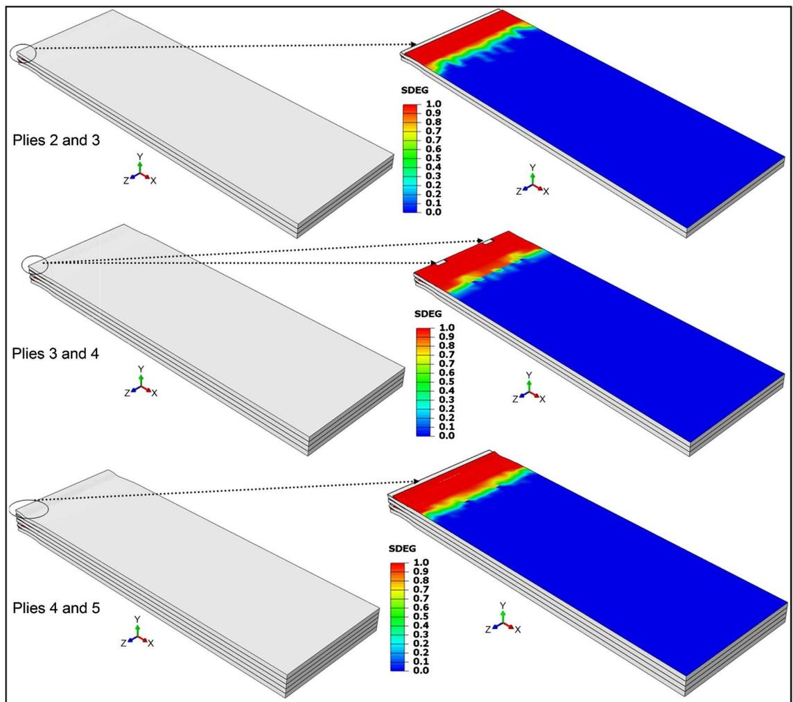
**Figure 9.** Contour plots showing the delamination in the standard modulus T300 composite under tension (elements were deleted upon reaching maximum degradation).
