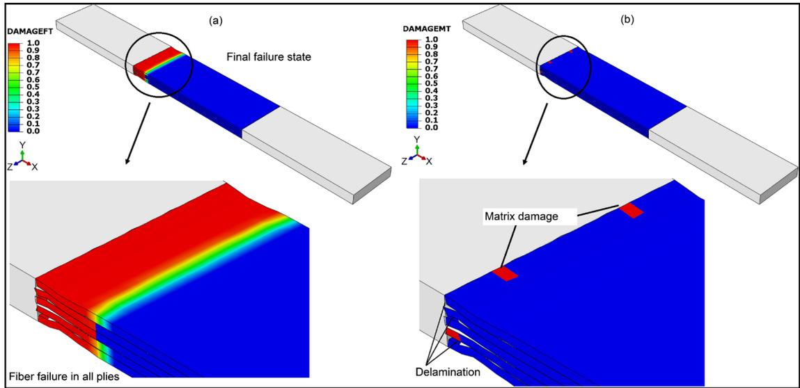
**Figure 8.** Contour plots (a), (b) of the fiber failure (DAMEGEFT), the matrix damage (DAMEGEMT) in the standard modulus T300 composite under tension at the final failure state.
