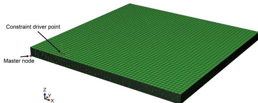
**Figure 3.** Assigning a constraint driver point within the unit cell for applying the uniaxial loads.
