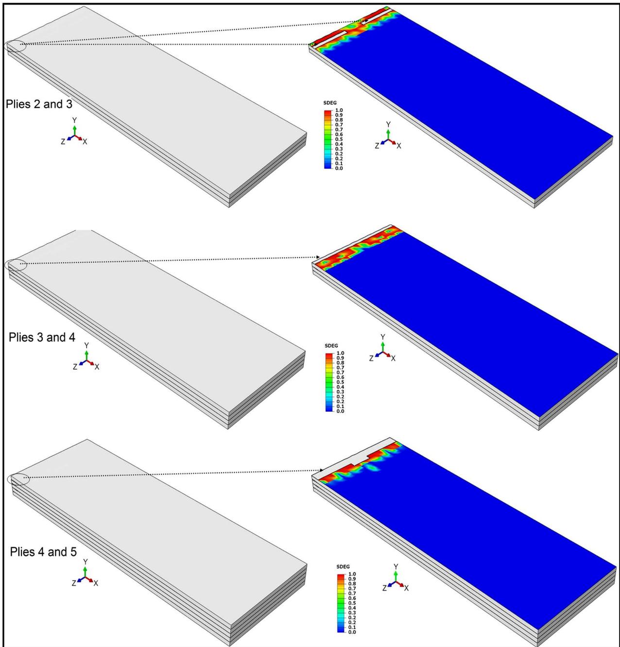
**Figure 13.** Delamination in the interface between the plies of the YS90A composite under tension.
