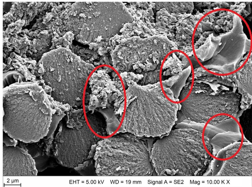
**Figure 10.** SEM image showing non-homogeneities in dispersion of DP (marked in red) in the composite.
