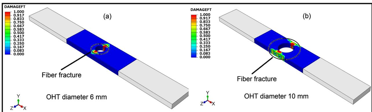
Figure 15. Fiber failure under tension for the YS90A composite with stress concentrations modeled with OHT coupons.
