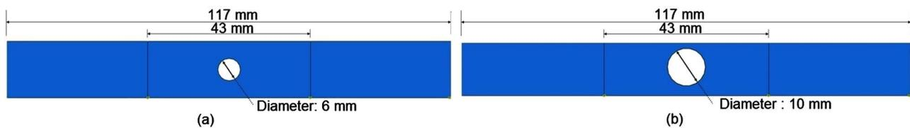
Figure 14. Development of the OHT laminate with a diameter of 6 mm (a) and 10 mm (b) for studying the behavior of stress concentrations under tensile loading.
