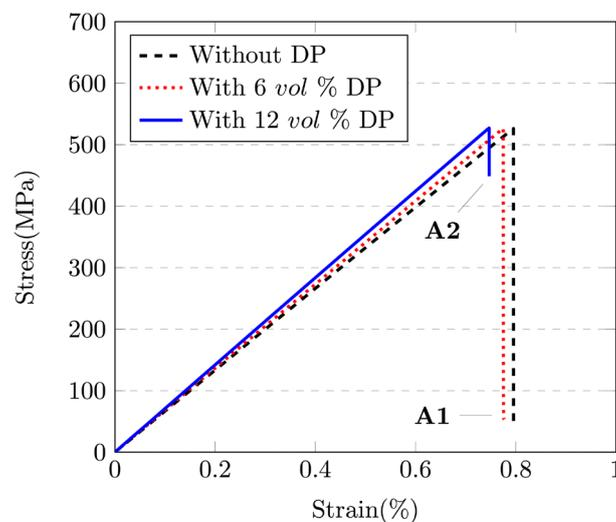
**Figure 7.** FEM results for the on-axis tensile behavior of T300-diamond powder epoxy filled composite.
