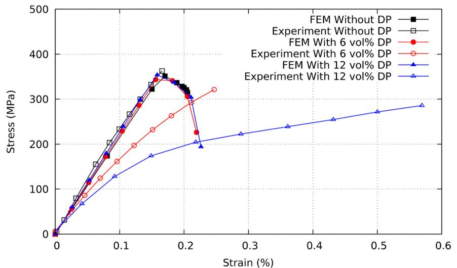
Figure 11. Comparison between the experimental tensile testing results and FEM tensile behavior without considering stress concentrations in the laminate.
