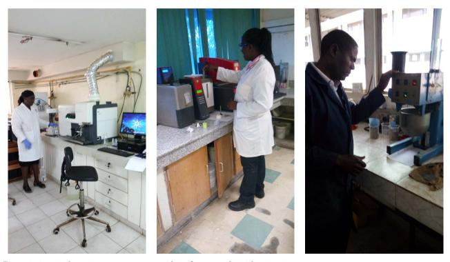
Figure 1. Atomic absorption spectrometer test, Blaine fineness and initial setting time test.
