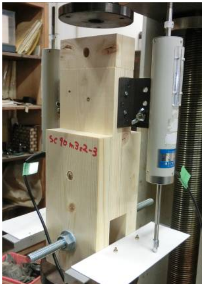
Figure 7. Double shear test setup, with load applied in direction parallel to the grain of the side member.
