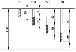
Figure 9. Positions of the thread on z-axis.
