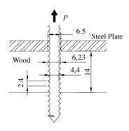
Figure 6. Cross-section of specimen.
