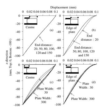
Figure 12. Displacement distribution by FEA.
