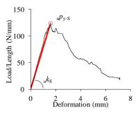
Figure 7. Determination of characteristic values of screw.
