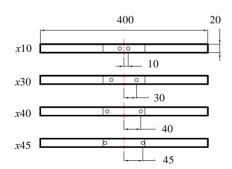
Figure 10. Positions of the thread in the x-axis.
