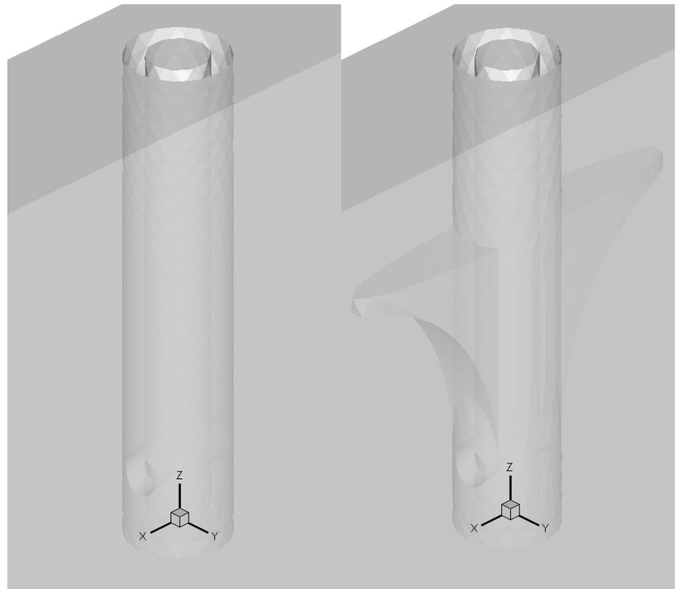
**Figure 1.** The conventional cylindrical SEN (left) and the anchor-shaped SEN (right).
