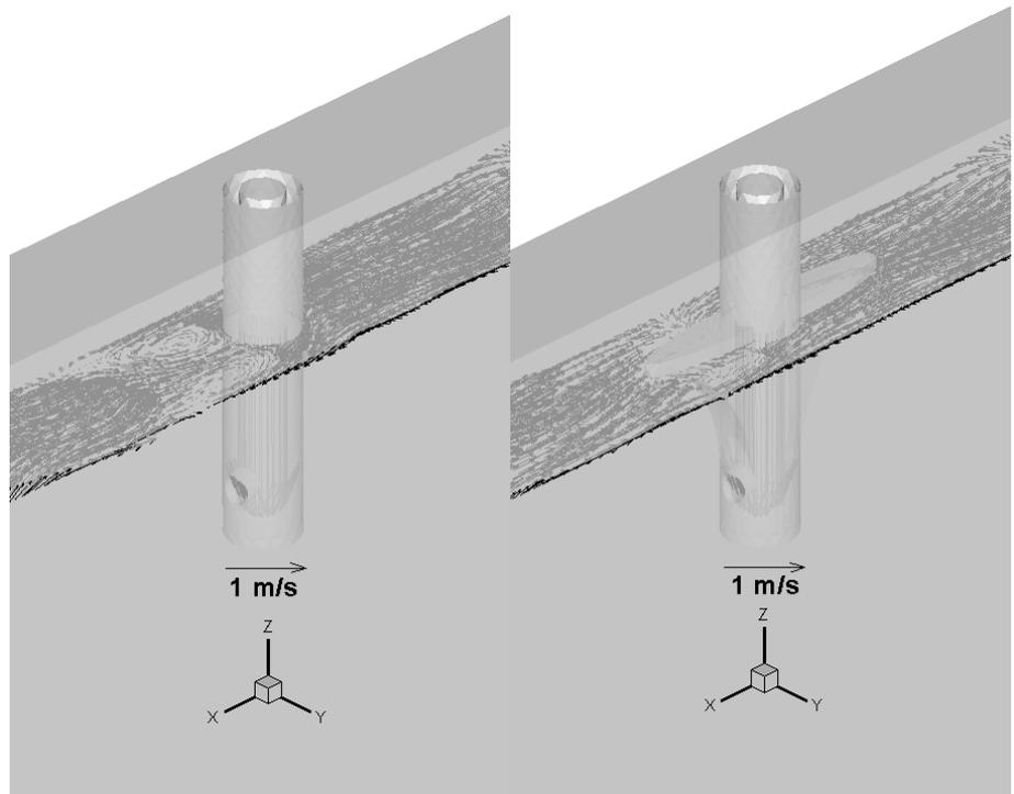
**Figure 5.** Velocity vectors in the horizontal plane  $Z = 0.8$ , close to the free surface. Cylindrical SEN (left), anchor-shaped SEN (right).
