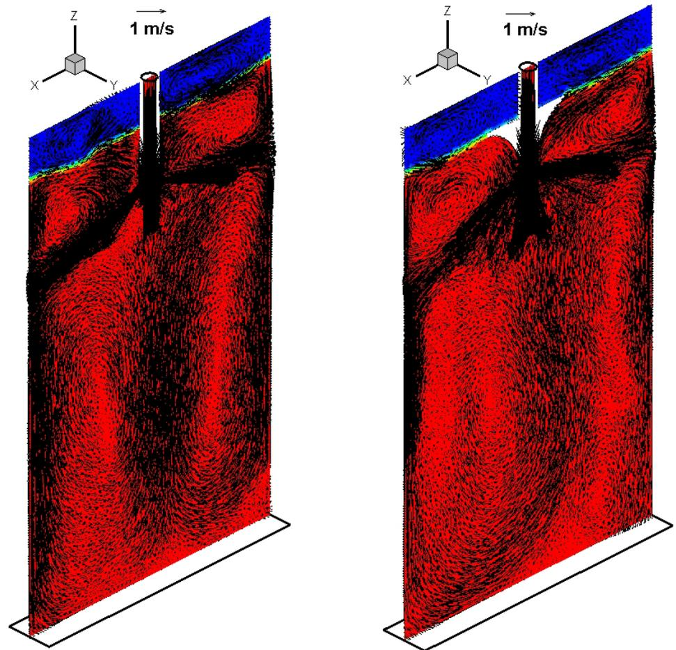
**Figure 3.** Phase distribution and velocity vectors for the conventional cylindrical SEN (left) and the anchor-shaped SEN (right) in the vertical plane  $Y = 0$ . Red phase is molten steel, blue phase is air. Elapsed time = 90 s.
