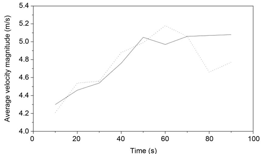
**Figure 6.** Evolution of the average velocity magnitude in the mold for the cylindrical SEN (solid line) and anchor SEN (dotted line).
