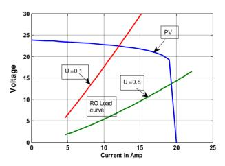
Figure 6. I-V curve and RO load curves for different valve positions.
