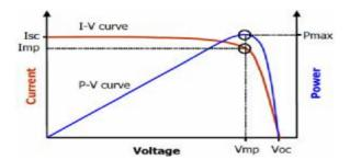
Figure 2. I-V and P-V curves of a typical PV array [5].
