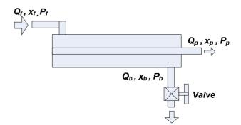
Figure 3. Illustration of the RO system.
