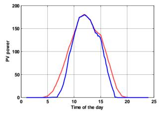
Figure 7. Dotted: available power; solid: used power.
