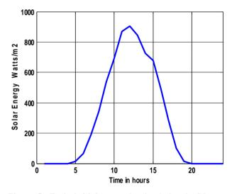
Figure 5. Typical 24 hours solar insolation in May at KFUPM.
