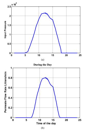
Figure 8. (a) Variation of Feed pressure (Pa); (b) Permeate water flow rate in L/min.
