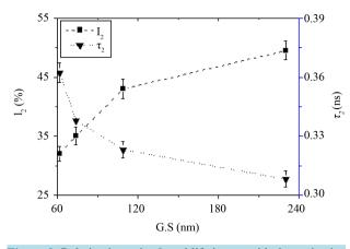
**Figure 2.** Relative intensity  $I_2$  and lifetime  $\tau_2$  with the grain size of Li-ferrite samples.
