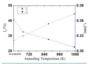
**Figure 1.** Relative intensity  $I_2$  and the lifetime  $\tau_2$  with the annealing temperature.
