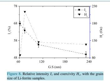
The novel point: the dominant factor for the decrease of  $H_c$  for G.S.  $\ge 109$  nm is the decrease of the intra granular pores of multi domains behavior. Meanwhile, the dominant factor for the increase of  $H_c$  for G.S. < 109 nm is the increase of inter granular pores for single domain nanograin Li-ferrite.
