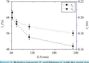
**Figure 4.** Relative intensity  $I_1$  and lifetime  $\tau_1$  with the grain size of Li-ferrite samples.
