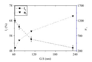
**Figure 6.** Relative intensity  $I_1$  and initial permeability  $\mu$  measured at 673 K with the grain size of Li-ferrite samples.
