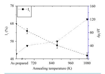
**Figure 7.** Relative intensity  $I_1$  and the homogeneity  $(\Delta \mu_i / \Delta T)$  with the annealing temperature of Li-ferrite samples.
