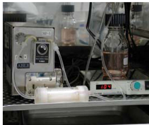
Figure 2. Specification and use method of the hollow fiber module. The hollow fiber module contains 394 hollow fibers, and the volumes of the inner space of the hollow fibers (lumen) and outer space (ECS) were 20 mL, respectively. There were two ports each connected to the lumen and ECS (4 ports in total). Culture medium was circulated through the ports connected to the lumen to grow cells in ECS. The external appearance (top), design (middle), and use (bottom) of the hollow fiber module were shown.
