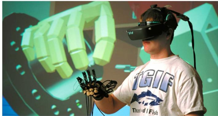
**Figure 4.** A head-mounted display with the tracking device flock-of-birds for telepresence in the immersive environment.
