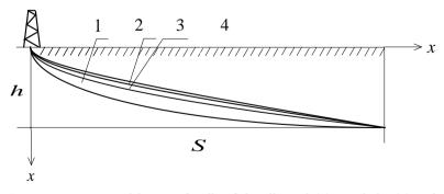
**Figure 1.** Geometrical layout of wells of the elliptical (1), parabolic (2) and hyperbolic (3, e = 1.01; 4, e = 1.015) shapes (h = 1000M, S = 4000M) {where the ellipse equation is  $S^2/a^2 + h^2/b^2 = 1$ , parabola:  $4pS = h^2$ , hyperbola:  $S^2/a^2 - h^2/b^2 = 1$ , *a*, *b*, and *p* are constants}.
