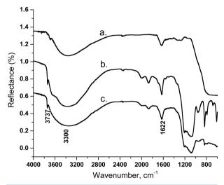
**Figure 3.** Infrared reflectance spectra of (a) TiO<sub>2</sub>-P25 (b) zeolite CBY780 and (c) Z-TiO<sub>2</sub> photocatalysts.
