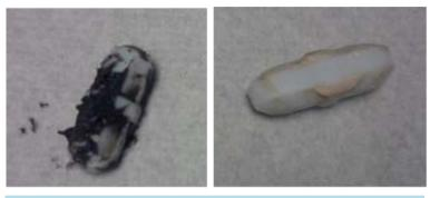
Figure 9. Appearance of stir bars from a mixture of Z-TiO<sub>2</sub> and naphthenic acid (Right) after exposure to UV light for 5 days and (Left) kept in dark for a week.
