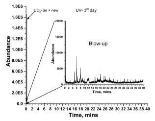
**Figure 8.** GC spectra of headspace gas from UV irradiation on Z-TiO<sub>2</sub> and naphthenic acid at 25°C over 3 days. Continued increase in CO<sub>2</sub> intensity. Inset: expanded region of the GC showing decline in abundance of the acid.
