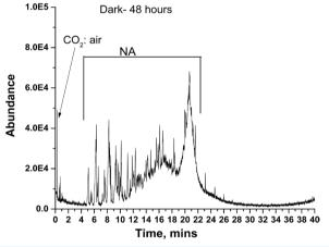
Figure 5. GC-MS spectra of head-space aliquots from mixture of Z-TiO<sub>2</sub> and naphthenic acid at 25°C kept in the dark for 48 hours.
