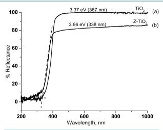
**Figure 2.** UV diffuse reflectance spectra of (a) TiO<sub>2</sub>-P25 (b) Z-TiO<sub>2</sub> photocatalysts.
