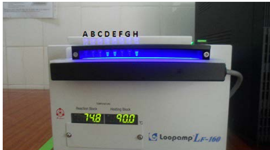
Samples A, B, C and F: fluorescence not detected ( M. tuberculosis strains not detected); Samples D and E: fluorescence detected ( M. tuberculosis strains detected); G: fluorescence not detected in Negative control tube; H: fluorescence detected in Positive control tube.
