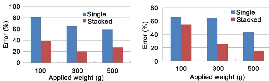
**Figure 5.** The error of the maximum (left) and minimum (right) convergent value apart from the average output voltage, respectively.
