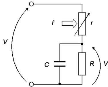
**Figure 1.** Detecting circuit of the output. The rubber sensor was indicated  $r$  in the figure.
