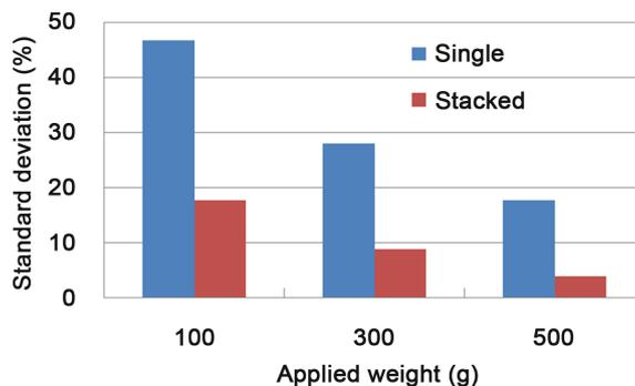
**Figure 6.** The standard deviation relative to the convergent average output voltage.
