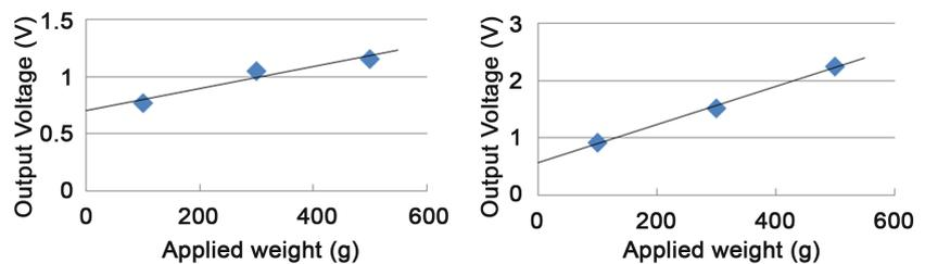
**Figure 4.** The average output voltage of the convergent value: a single sensor (left) and a stacked sensor (right).
