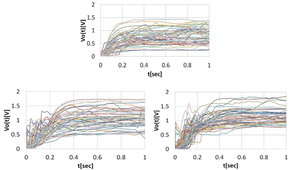
**Figure 2.** The transient output voltage of 50 trials for a single sensor. The applied load was 100 g (top-left), 300 g (bottom-left) and 500 g (bottom-right), respectively.
