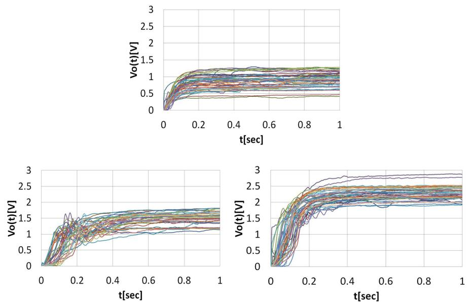
**Figure 3.** The transient output voltage of 50 trials for a stacked sensor. The applied load was 100 g (top-left), 300 g (bottom-left) and 500 g (bottom-right), respectively.
