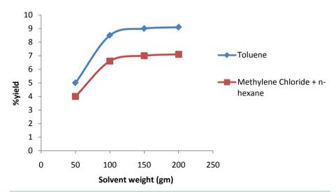
Figure 4. Effect of solvent to oil shale ratio.
