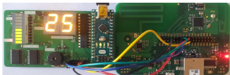
Figure 7. The silo industrial automation thing based on a hardware silo simulator.
