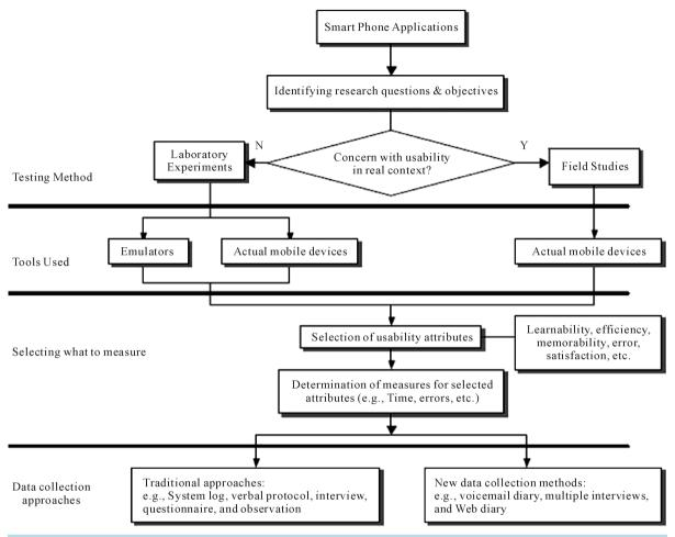
Figure 1. A structure for design and implementation of usability testing of smart phone applications.
