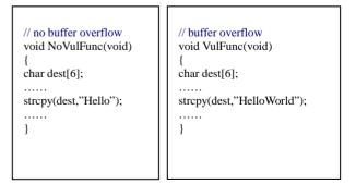
Figure 1. An example of a buffer overflow.
