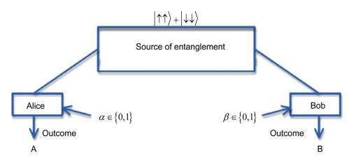
**Figure 2.** The operation principle of the proposed QKD protocol. An entanglement source produces a pair of entangled signals, which are randomly measured in certain bases chosen by Alice and Bob separately. Alice and Bob generate outcomes *A* and *B* respectively.
