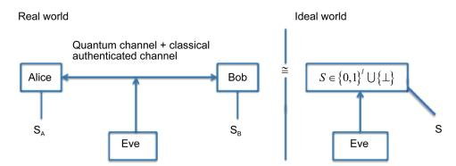
**Figure 1.** Comparison between what happens in a real and ideal quantum cryptographic world. Alice and Bob use the quantum and classical authenticated channel in the presence of Eve. At the end of communication; in the real world, Alice and Bob share two correlated secret keys  $S_A$  and  $S_B$ , respectively. In an ideal world, the access of Eve is broken; therefore Alice and Bob share a perfect secret key *S*.
