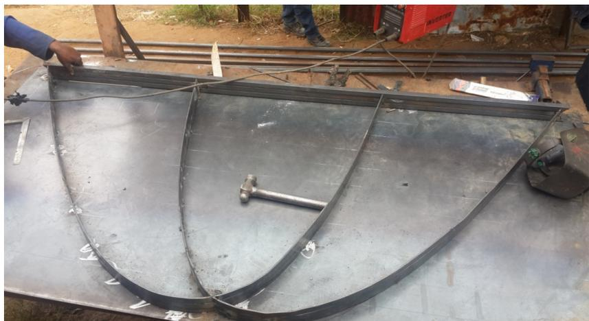
**Figure 8.** Constructing the four wing CPC profile on a sheet metal base.
