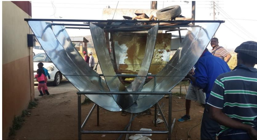
**Figure 9.** Construction of the wings, frame, absorber and reflector surfaces.
