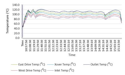
Figure 5. Collector field temperature distribution.
