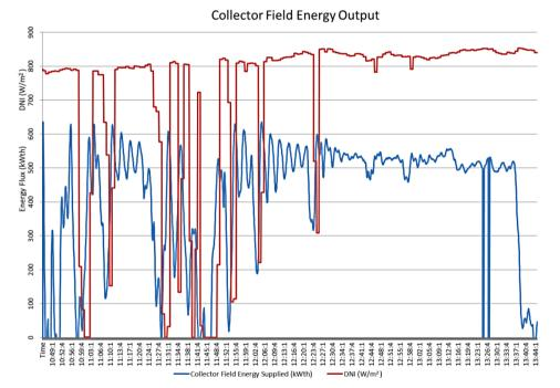
Figure 7. Collector field energy output, day 2.
