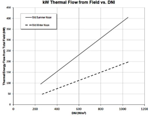
Figure 2. Collector field output vs. DNI. Source: 3 M.
