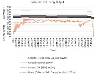
Figure 6. Collector field energy output.
