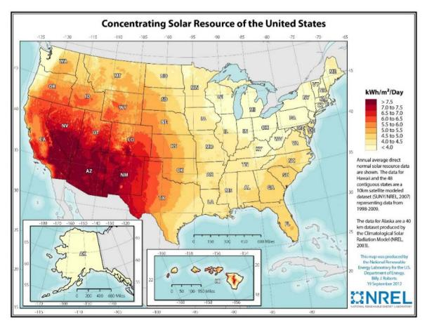
Figure 1. Concentrating solar resource of the US source: National renewable energy laboratory solar data center.
