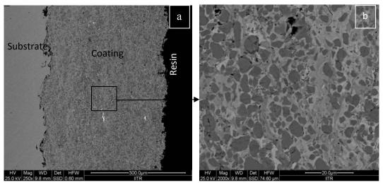
Fig.4. BSEI micrograph showing cross-section morphology of HVOF sprayed 75Cr<sub>3</sub>C<sub>2</sub>-25NiCr coating on T91boiler steels in as-sprayed condition.
