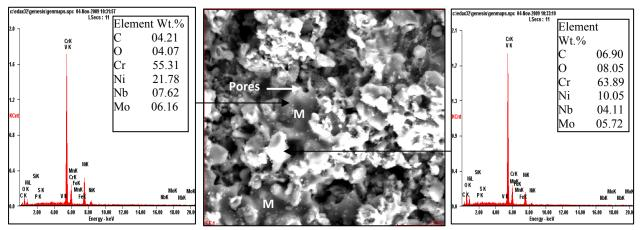
Fig.5. SEM micrograph and EDAX analysis surface of HVOF sprayed 75Cr<sub>3</sub>C<sub>2</sub>-25NiCr coating on T91 substrate.
