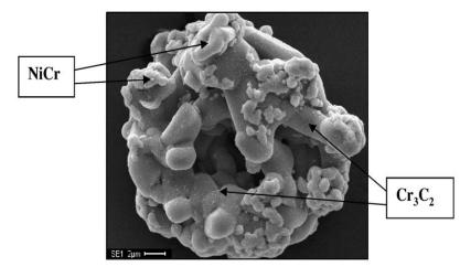
Fig.2. FE-SEM of Cr<sub>3</sub>C<sub>2</sub>-NiCr powder particle [3]
