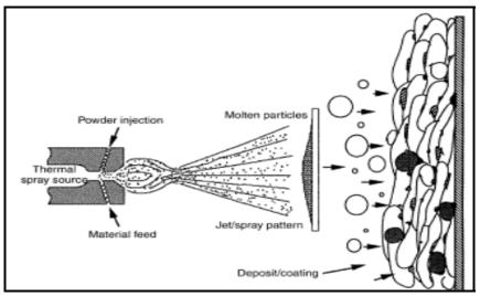
Fig.1.Typical thermal spray process and coating [1]
