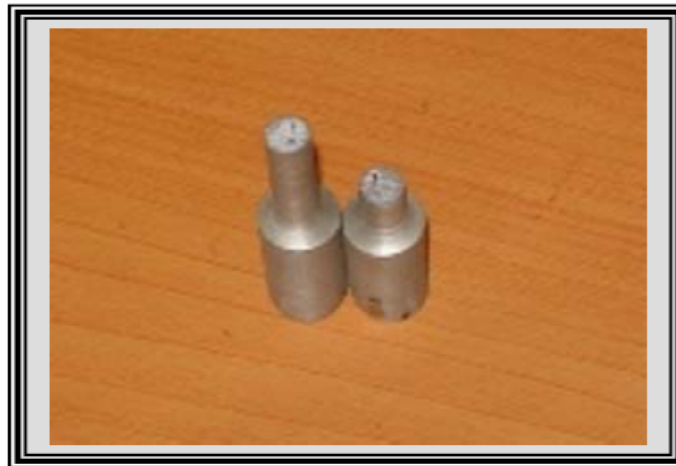
Figure (7) Good bonding in the specimen squeeze cast at T_p = 700^\circ C , T_d = 200^\circ C and P = 53 MPa .
