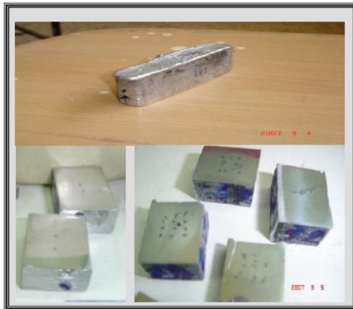
Figure (3) Some of the squeeze cast specimens.
