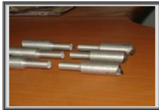
Figure (5) Some of the tensile tested specimens.
