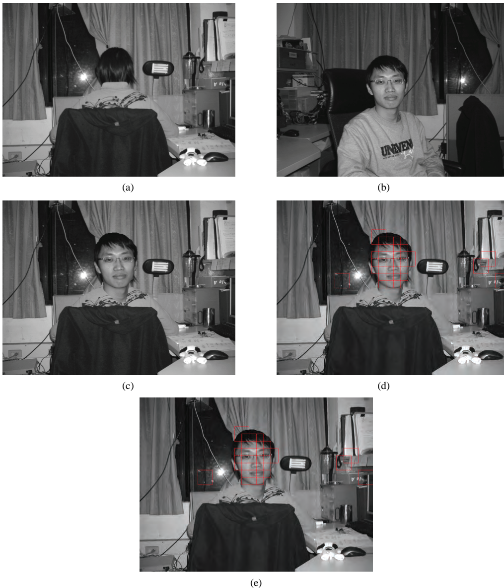
Figure 15. (a) Original image; (b) Image with up-sample rate 5%; (c) Forgery image composed from (a), (b); (d) Detection result with 64 \times 64 block size; (e) Detection result with 128 \times 128 block size.
