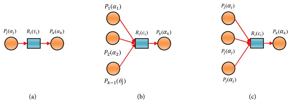
**Figure 1.** FRSN P systems rule neurons. (a) A general rule neuron,  $\alpha_k = \alpha_j * \tau_i$ ; (b) And rule neuron,  $\alpha_k = \min\{\alpha_1, \alpha_2, \dots, \alpha_{k-1}\} * \tau_i$ ; (c) Or rule neuron,  $\alpha_k = \max\{\alpha_1, \alpha_2, \dots, \alpha_{k-1}\} * \tau_i$ .
