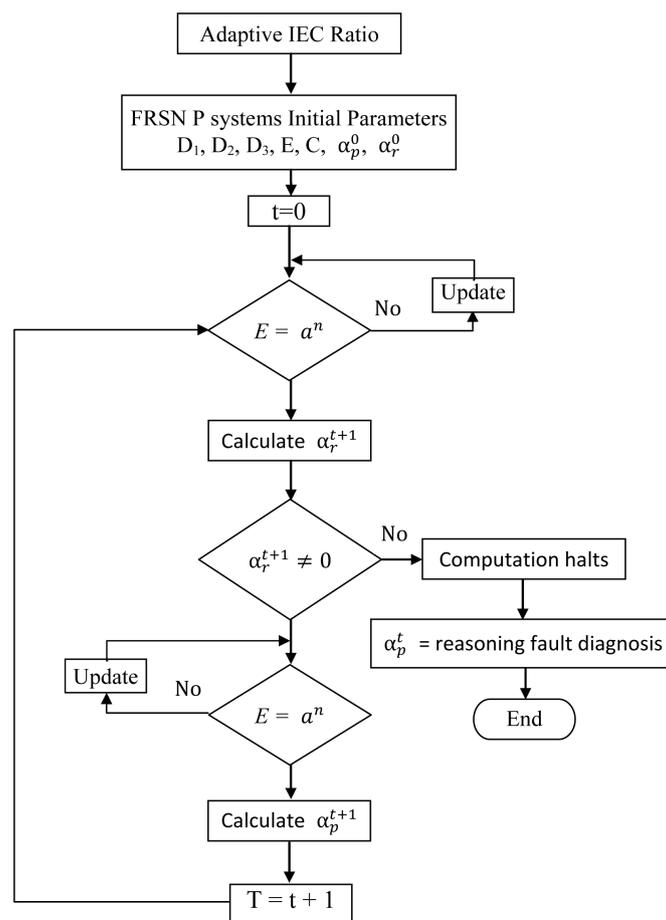
**Figure 3.** FRSN P systems transformer fault diagnosis flow chart.
