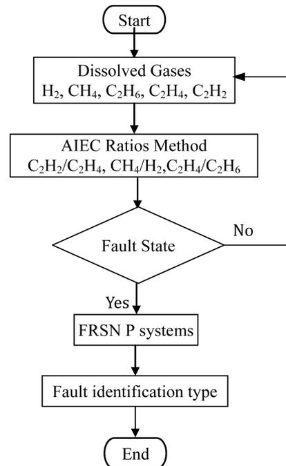
**Figure 2.** Transformer fault diagnosis based on DGA & FRSN P systems.
