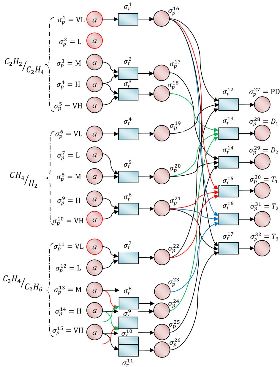
Figure 4. FRSN P systems fault diagnosis graphical model.
