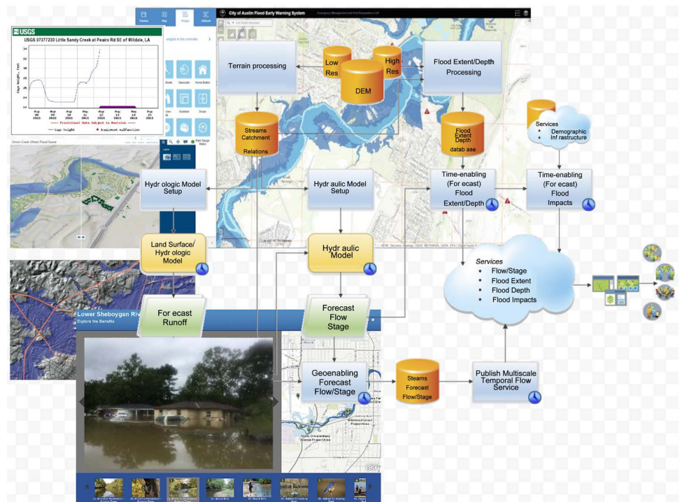
Figure 7. Integrating geospatial analytics, visualization and machine learning into WaVE’s common operating picture framework and decision support toolset. Images courtesy of Esri.
