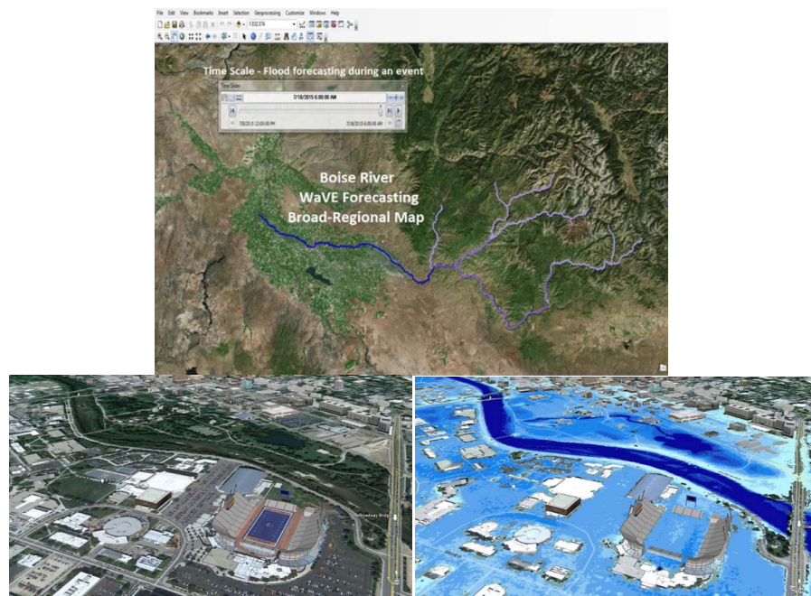
Figure 10. Plates demonstrating WaVE forecast and pre and post flood inundation in downtown Boise. Images courtesy of Esri and designed using ArcGIS 10.3 and Arc Hydro and Google Map services.
