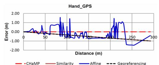
**Figure 4. Relative error in point positions using Gamin GPS control points.**
