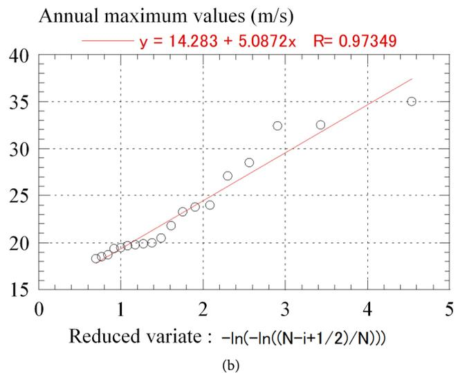
**Figure 10.** Relationship between the annual maximum values of the 10-minute average wind speed data collected at the Wakayama Meteorological Observatory and the reduced variate of the Gumbel analysis. (a) For the entire range of wind speeds (=47 data values); (b) For the high wind speed range (wind speeds equal to or larger than 19 m/s).
