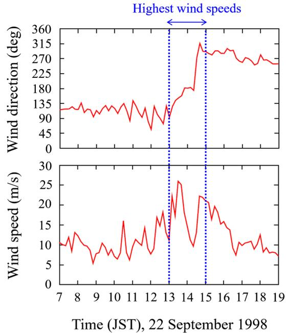
**Figure 5.** Time series of wind direction and speed at observation pole No. 2 at the wind farm under investigation on September 22, 1998. The wind directions 0, 90, 180, and 270 degrees represent northerly, easterly, southerly, and westerly winds, respectively.
