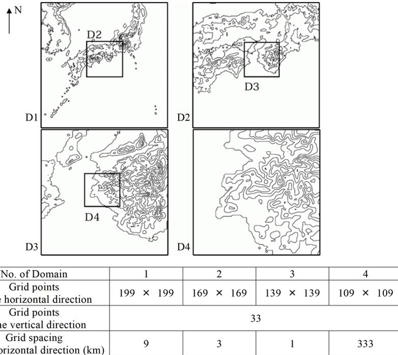
**Figure 3.** Computational domain and model terrain used in the MM5 mesoscale model.
