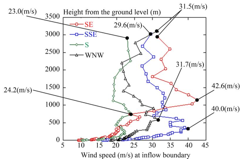
**Figure 9.** Results of the typhoon simulations: vertical profiles of the horizontal wind speed at the center of the inflow boundary of the computational domain from the time of the largest simulated value of the horizontal wind speed at observation pole No. 2. The wind profiles are plotted for the south-easterly, south-south-easterly, southerly, and west-north-westerly wind cases.
