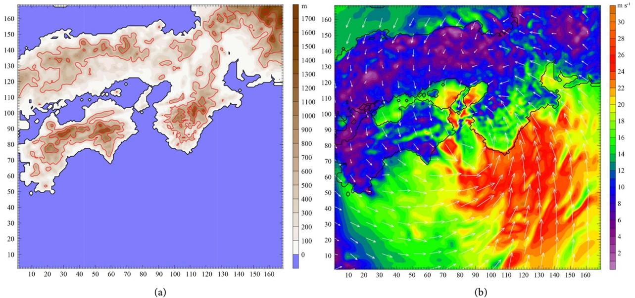
**Figure 6.** Distribution of the horizontal wind vectors from the lowest layer in Domain 2, approximately 11 m above the ground surface. 1330 LST, 22 September, 1998. (a) Topography; (b) Horizontal wind vectors.
