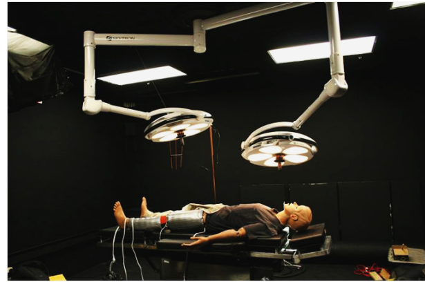
Figure 1. Full-scale laboratory chamber used for evaluation of air distribution via flow visualization and PIV.
