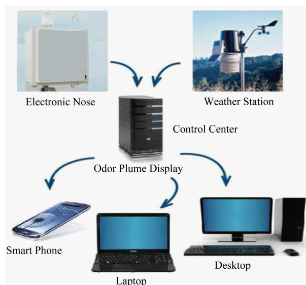
Figure 1. The architecture of continuous monitoring system of odors installed.
