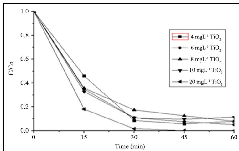
**Figure 2.** Comparison of the photodegradation efficiency of  $1 \text{ mg}\cdot\text{L}^{-1}$  of IBF with variation of the catalyst concentration. Irradiation source 125 W Hg vapor lamp, aerated solution; pH 7.8; total solution volume: 500 mL.
