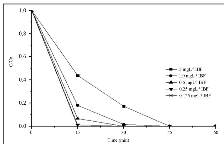
**Figure 3.** Comparison of the photodegradation efficiency at different IBF initial concentrations, using 20 mg·L<sup>-1</sup> TiO<sub>2</sub> (P25). Irradiation source: 125 W Hg vapor lamp, aerated solution; pH 7.8; total solution volume: 500 mL.
