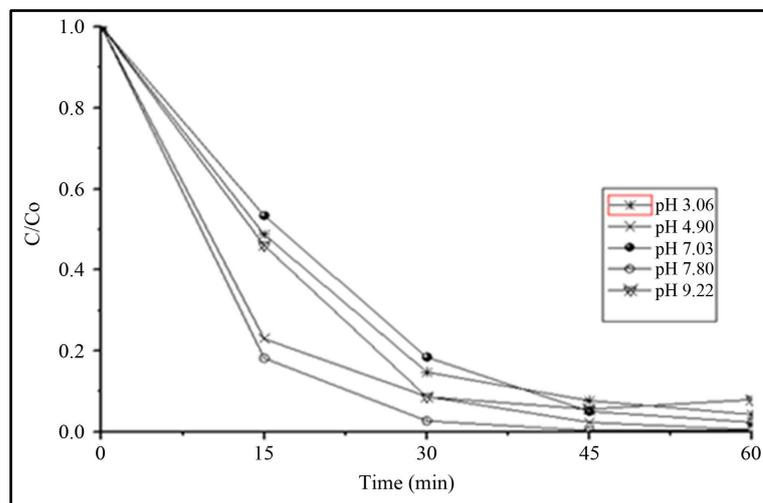
**Figure 1.** Comparison of the pH variation in the efficiency of the photodegradation study of  $1 \text{ mg}\cdot\text{L}^{-1}$  of IBF using  $4 \text{ mg}\cdot\text{L}^{-1}$  of  $\text{TiO}_2$ . Irradiation source 125 W Hg vapor lamp, aerated solution; total solution volume: 500 mL.
