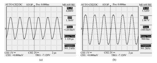
Figure 5. Waveform and electrical parameters of the TCA on frequency 300 kHz. (a) 4 Vpp, (b) 5.3 Vpp.
