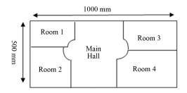
Figure 2. A Residential Building-like Test-bed.
