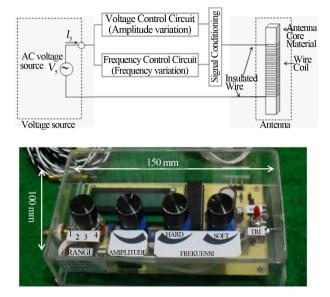
Figure 1. The Developed Termites Control Apparatus.
