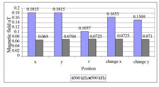
Figure 7. Magnetic field from TCA with frequencies 300 kHz and 500 kHz.
