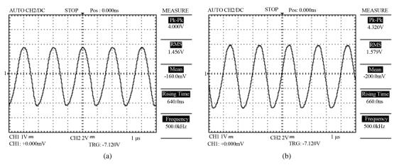
Figure 6. Waveform and electrical parameters of the TCA on frequency 500 kHz. (a) 4 Vpp, (b) 4.3 Vpp.
