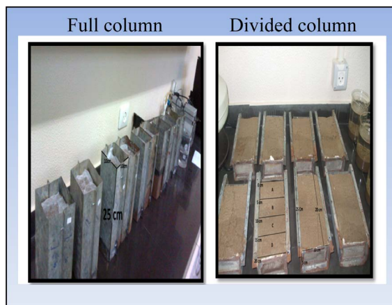
Figure 2. Column technique used for HPLC and bioassay techniques for determination of leaching potential in soil. Left photo shows full column filled with sandy soil and treated with chlorpyrifos and irrigated with water. Right photo shows the columns split lengthwise to form 2 pots.
