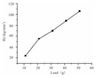
Figure 3. Vickers hardness profile of L-phenylalanine-4-nitrophenol as a function of applied load.
