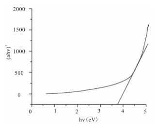
Figure 2. Plot of  $(\alpha h v)$ 2 versus h v for L-phenylalanine-4nitrophenol single crystal.
