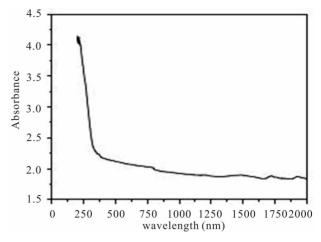
Figure 1. Transmission spectrum of L-phenylalanine-4nitrophenol crystal.
