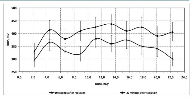
**Figure 2.** Change of water ORP value under  $\alpha$ -irradiation.
