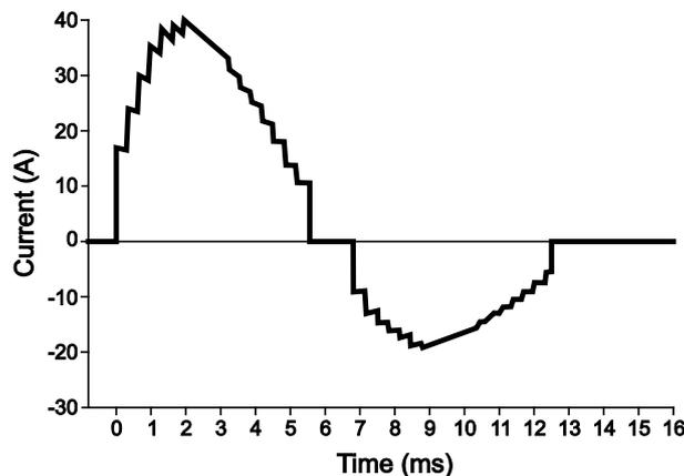
**Figure 3.** Biphasic stepwise asymmetric quasi-sinusoidal pulse waveform (“DKI-N-02 St” current-based defibrillator, current amplitude 40 A, TTI 50  $\Omega$ , energy 200 J).
