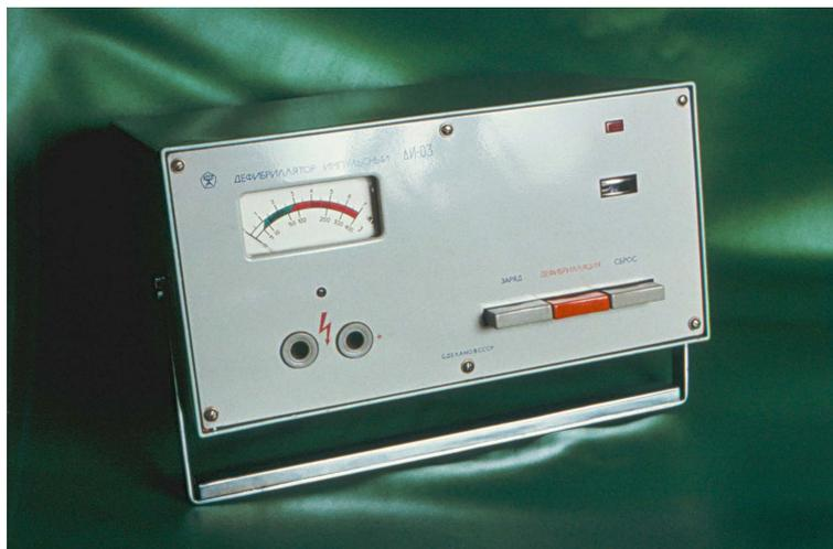
**Figure 1.** The world’s first biphasic waveform defibrillator DI-03 (USSR, 1971).
