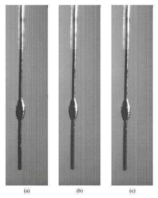
**Figure 5.** A sequence of photographs extracted at 2-second intervals from high-speed photography for operation with a concentric 2.5 mm crown rotating at 214,000 rpm.
