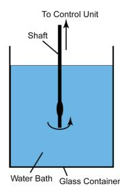
Figure 2. Diagram of the experimental setup with the atherectomy device situated in the vertical orientation in a large water environment.
