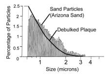
**Figure 4.** Particle size distributions for the dispersed sand and debulked plaque.
