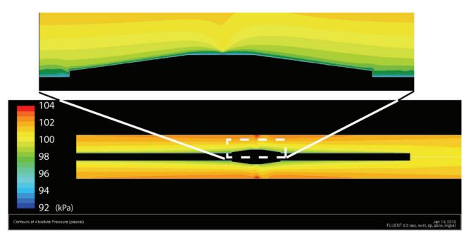
Figure 9. Variation of the pressure in the vicinity of the rotating atherectomy device positioned within a tube.
