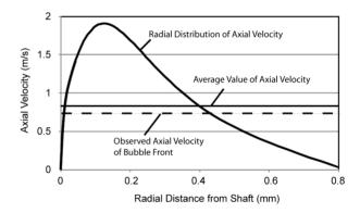
Figure 11. Comparison of observed and calculated axial velocity results upstream of the rotating crown. The horizontal lines represent local-averaged velocities, respectively from the numerical simulations and from the visual observations.
