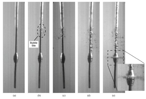
Figure 7. A sequence of photographs extracted at 2-second intervals from high-speed photography for operation with a concentric 2.5 mm crown rotating at 214,000 rpm and with introduced air bubbles serving as a tracer.
