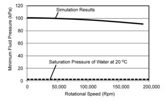
Figure 8. Variation of the minimum pressure caused by rotation of the atherectomy device in a tube.
