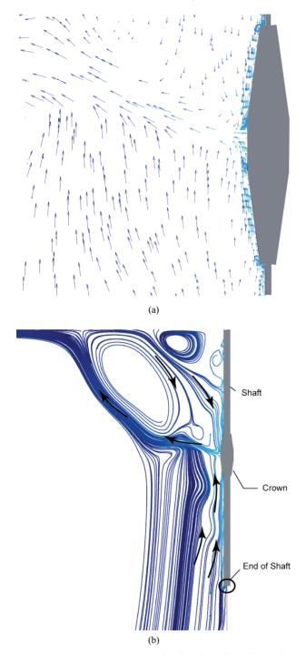
**Figure 10.** (a) Vectors showing the direction of the flow adjacent to the crown of a rotating atherectomy device situated in a water bath; (b) Streamlines of the flow adjacent to the crown of a rotating atherectomy device situated in a water bath.
