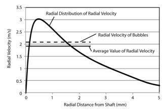
Figure 12. Comparison of observed and calculated radial velocity results at the apex of the rotating crown. The horizontal lines represent local-averaged velocities, respectively from the numerical simulations and from the visual observations.
