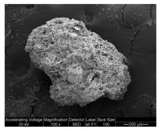
Figure 4. SEM appearance of a typical pumicite grain.
