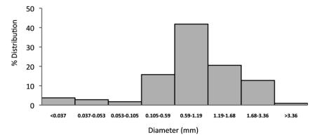
Figure 2. Grain-size-distribution curve. In the figure the percent size distribution is plotted *versus* the grain diameter in mm.
