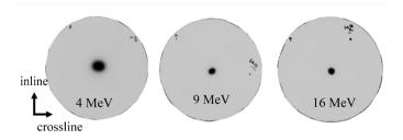
**Figure 4.** Two-dimensional optical density distribution of radiochromic film irradiated by (a) 4, (b) 9, and (c) 16 MeV electron beams.
