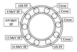
**Figure 1.** Position of scattering foils for different energies [10] and flattening filters on carousel of medical linear accelerator.
