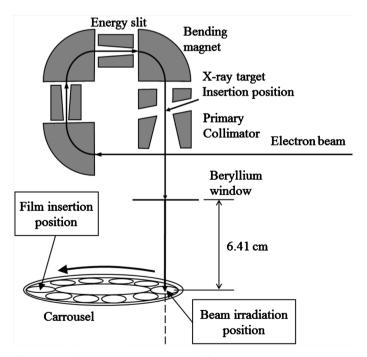
**Figure 2.** Film insertion position and beam irradiation position on carrousel in medical linear accelerator gantry head [9].
