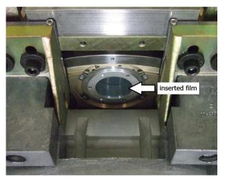
**Figure 3.** Picture of scattering foil bracket with MD-55 radiochromic film at "film insertion position" shown in **Figure 2**.
