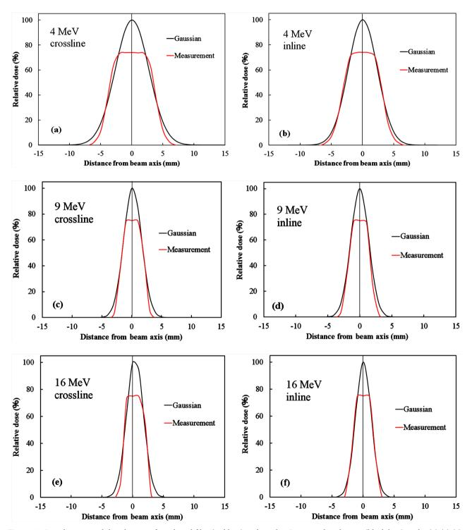
**Figure 5.** One-dimensional distribution of irradiated film (red line) and similar Gaussian distribution (black line) in the (a) (c) (e) crossline and (b) (d) (f) inline direction for beam energies of (a) (b) 4, (c) (d) 9 and (e) (f) 16 MeV.
