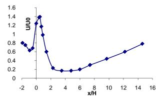
**Figure 6.** Velocity distribution across a model shrub; H and x are the height of shrub and distance from it, respectively; U0 is far upstream velocity and U is velocity at distance x.
