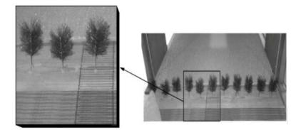
Figure 4. Experimental setup showing the erection of pro-typed shrub models across the test-section of the wind tunnel.
