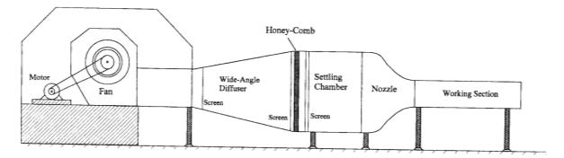
Figure 3. Components of Kuwait Institute for Scientific Research (KISR) wind tunnel.
