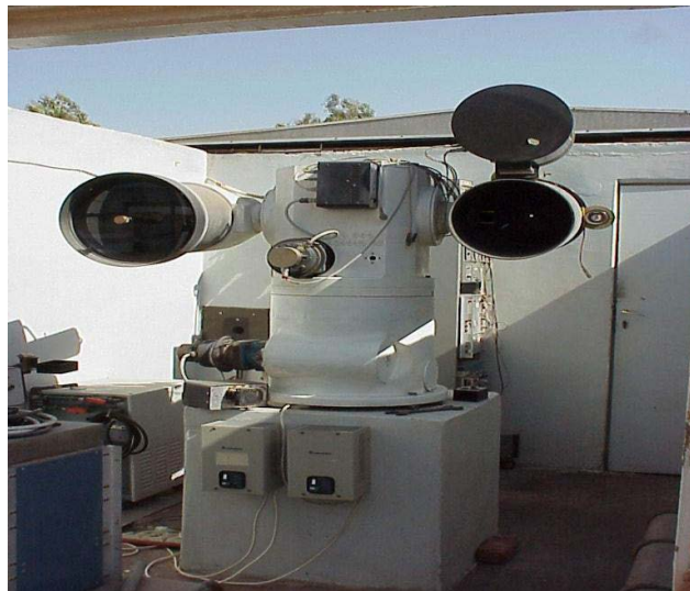
Figure 3. Helwan SLR station.
