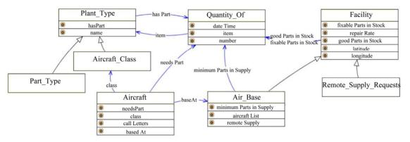
Figure 4. Partial aircraft entity relationship diagram and its attributes.
