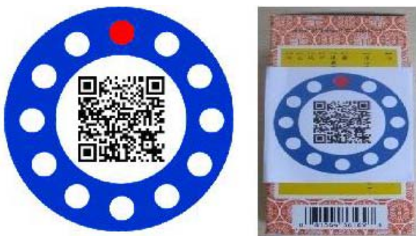
Figure 2. QR code model, on the left is artificial landmark based on QR code, on the right is object sticking with QR code.
