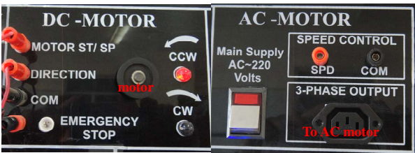
Figure 11. DC and AC motor drivers' connection.
