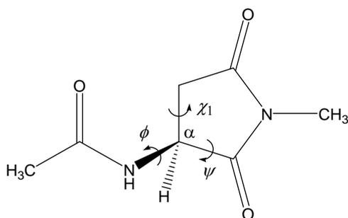
**Figure 2.** Model compound used in the present study (Ace-Asu-Nme). The dihedral angles  $\phi$  (C-N-C $_{\alpha}$ -C) and  $\psi$  (N-C $_{\alpha}$ -C-N) characterize the main-chain conformation.
