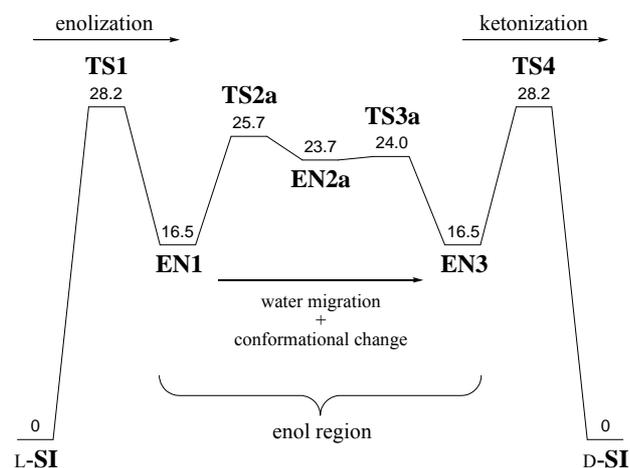
**Figure 4.** Energy diagram. ZPE-corrected energies relative to L-SI are shown in kcal·mol<sup>-1</sup>.
